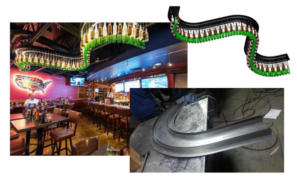
A sheet metal chandelier created for Red Robin restaurants. Each individual arc segment is modular, allowing them to be "chained" to fill a longer space. It was gratifying to hear that my tab/slot design "just fell together on the welding table."
