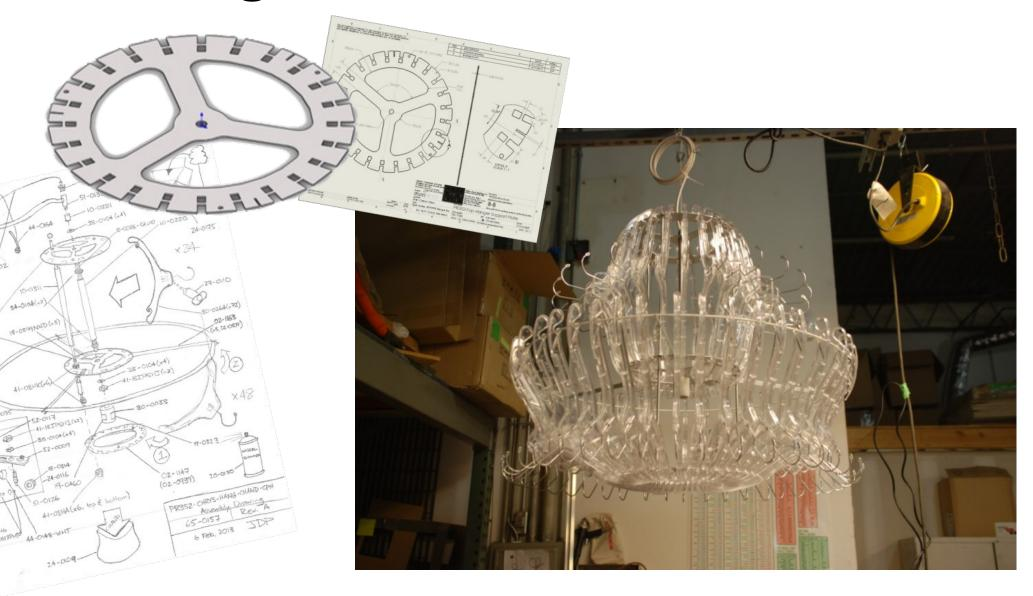
The original design for this fixture called for a heavy & expensive welded steel frame. After some experimentation, I developed a system of interlocking plates that reduced the overall weight to 10 lbs. & required only 3 tack welds. I was proud of the customer's enthusiasm for the new design.
